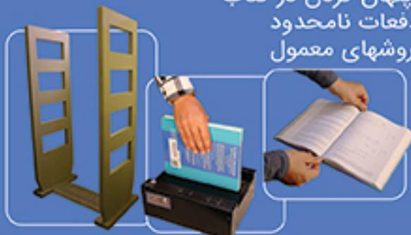
A tag is an electronic article placed on books, magazines, paper documents or CDs which are supposed to be protected by library security systems. one of the most important quality of EM tags is their capability of being activated and reactivated for numerous times .Obviously for reference books or documents that are never lent, permanent active tags are used.
